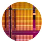
**SRAM** : 1 bit = 6 transistors
