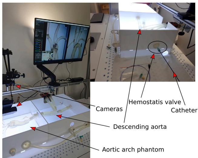
Fig. 1. Overview of the phantom aorta test bench used at BCV.
