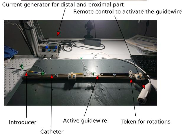
Fig. 3. Additional set-up to measure clinician movements during navigation: instrumentation of the BCV bench.
