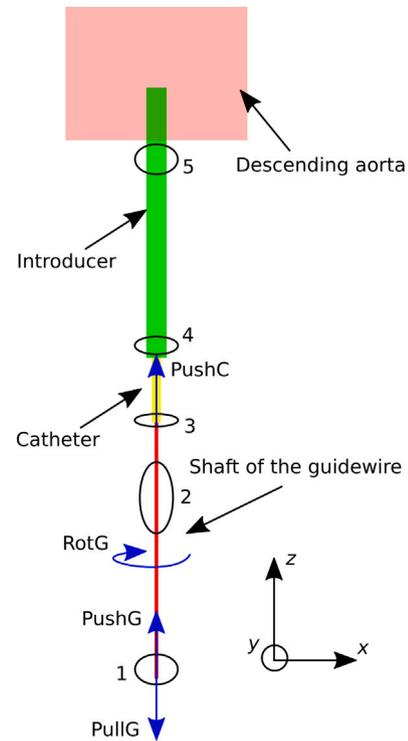
Fig. 5. Boundary conditions applied on the devices during endovascular navigation. PushC, PushG, PullG and RotG are related to Table 1 defining the different movements and their value.
