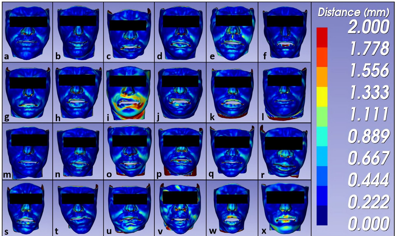
FIGURE 9 | Color map showing the Euclidean distance between the generated patient FE meshes and the corresponding real patient 3D surfaces.
