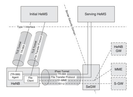
Figure 13.7 Example deployment of initial and serving HeMS.
