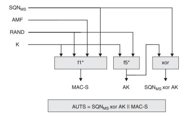
**Figure 7.4** Construction of the parameter AUTS. (Adapted with permission from © 2009, 3GPP<sup>TM</sup>.)
