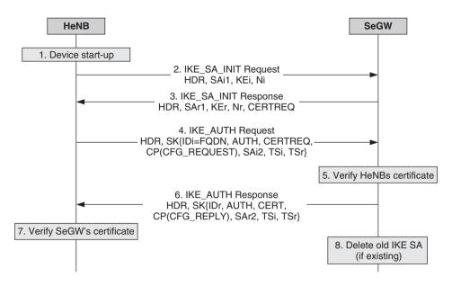
**Figure 13.3** Certificate-based authentication with device integrity validation. (Adapted with permission from © 2010, 3GPP<sup>TM</sup>.)
