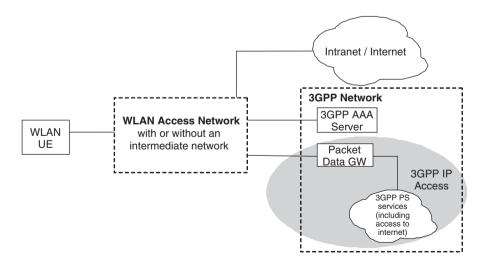
Figure 5.3 Simplified WLAN network model. (Adapted with permission from © 2009, 3GPP<sup>TM</sup>.)
