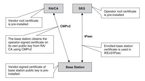
**Figure 8.5** Overview of security architecture for base station enrolment. (Adapted with permission from © 2010, 3GPP<sup>TM</sup>.)
