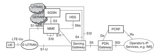
**Figure 2.2** The EPS architecture (nonroaming case). (Adapted with permission from © 2009, 3GPP<sup>TM</sup>.)
