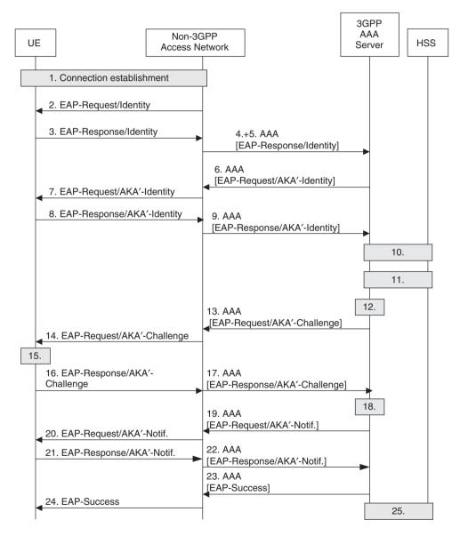
Figure 11.1 EAP AKA' authentication for trusted non-3GPP access.
