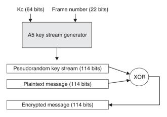
Figure 3.4 GSM encryption.
