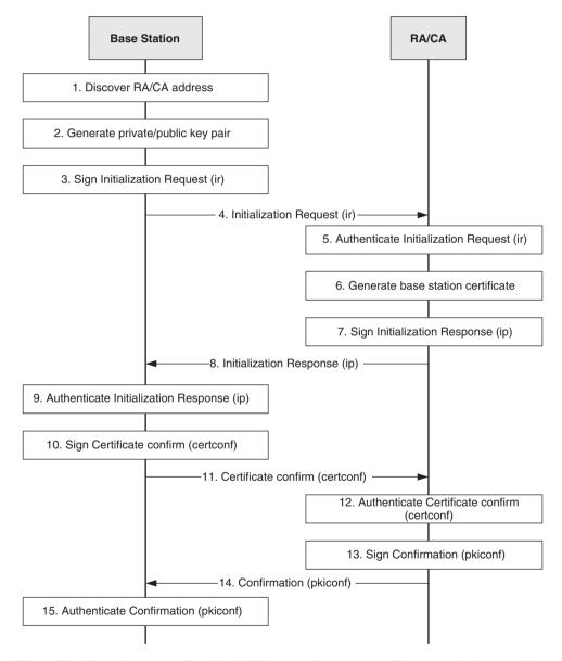
**Figure 8.6** Example message flow for initial base station enrolment. (Reproduced with permission from © 2010, 3GPP<sup>TM</sup>.)
