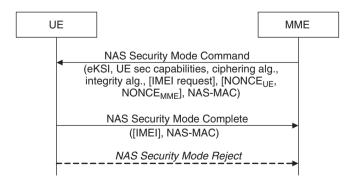
Figure 8.1 NAS Security Mode Command procedure.
