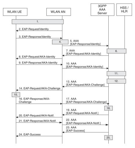
Figure 5.4 USIM-based authentication and authorization for direct IP access. (Adapted with permission from © 2010, 3GPP<sup>TM</sup>.)
