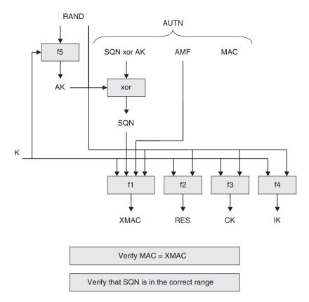
**Figure 7.3** User authentication function in the USIM. (Adapted with permission from © 2009, 3GPP<sup>TM</sup>.)
