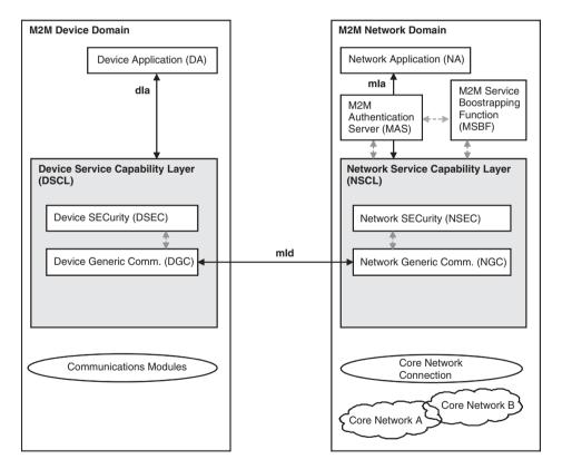
**Figure 15.1** Functional architecture elements for automated bootstrapping. (©European Telecommunications Standards Institute 2011. Further use, modification, copy and/or distribution are strictly prohibited. ETSI standards are available from http://pda.etsi.org/pda/).
