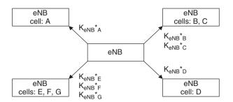
Figure 9.5 Separate keys for different target cells.
