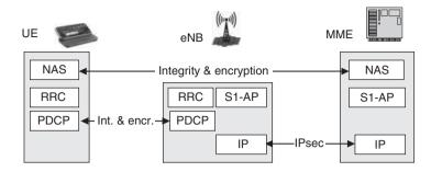
Figure 6.2 EPS signalling plane protection.
