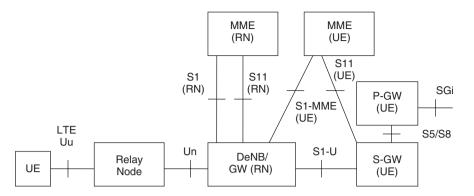
Figure 14.2 Relaying architecture in LTE. (Adapted with permission from © 2012, 3GPP<sup>TM</sup>.)
