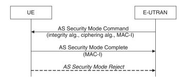
Figure 8.2 AS Security Mode Command procedure.
