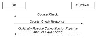
**Figure 9.6** eNB periodic local authentication procedure. (Reproduced with permission from © 2010, 3GPP<sup>TM</sup>.)
