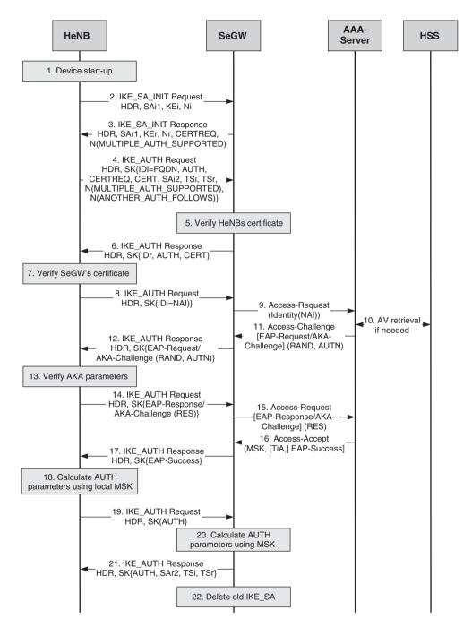
Figure 13.4 Device and hosting party identity-based authentication. (Adapted with permission from © 2010, 3GPP<sup>TM</sup>.)
