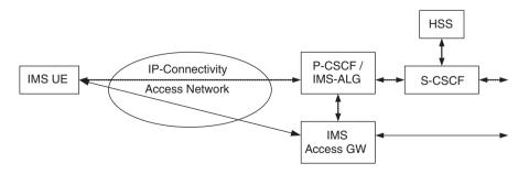
Figure 12.1 Partial view of the IMS architecture.
