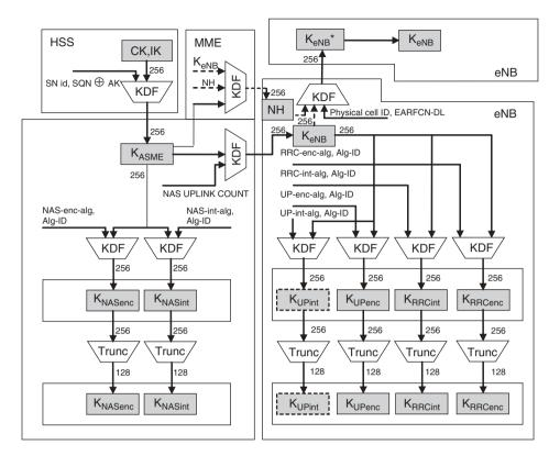
Figure 7.6 EPS key derivations on network side. (Adapted with permission from © 2010, 3GPP<sup>TM</sup>.)
