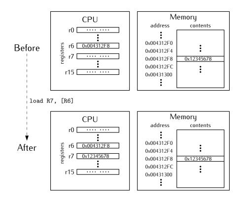
**ASM syntax and binary encoding** (This section is for reference only. Skip it on your first read). Both memory transfer instructions use **register-indirect** addressing: the address of the desired memory location is given by a CPU register, e.g. [R6] in the example on the preceding page. In our ASM syntax, a memory operand is always surrounded with square brackets.
