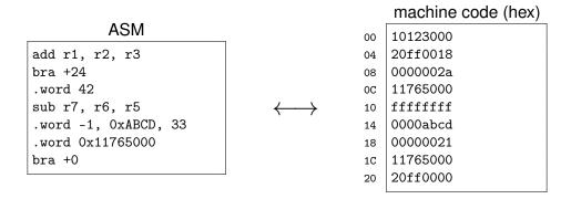
**Symbolic labels for data** In the previous chapter, we saw that named labels can be associated with program locations. Labels can actually be used to reference any location in memory, whether this location contains a program instruction or a piece of data. This is very useful to declare named constants or global variables, for instance "var: .word 0xff241300".
