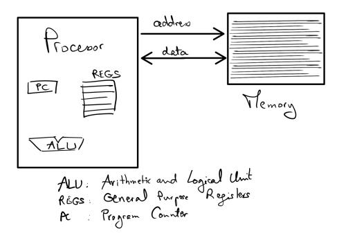
**The von Neumann principle** (aka stored-program concept) refers to the idea of representing both data and program instructions as bits stored in memory. The CPU implements the following behaviour known as the **von Neumann cycle**:
