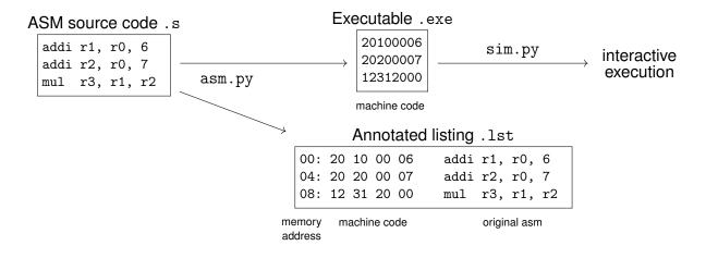
**Exercise** Type python3 scat/sim.py first.exe to invoke the simulator. By default, the simulator shows the contents of every CPU register, as well as an exerpt from the annotated listing with the next instructions that will be executed. Type step to execute just one instruction. Observe that this changes the values of registers, and that we "advance" in the program. Continue execution until the program is finished (try to predict the effect of each instruction).
