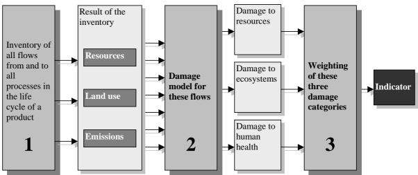
Figure 6: General procedure for the calculation of Eco-indicators. The light coloured boxes refer to procedures, the dark coloured boxes refer to intermediate results.
