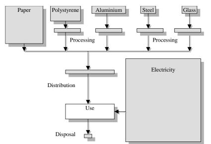
*Figure 4: The coffee machine process tree, where the size of the process blocks is proportional to the relative importance of the process.*
