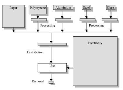
(graphical representation of the results of an Eco-indicator analysis of a coffee machine; the size of the boxes indicates the relative contribution to the environmental load)
