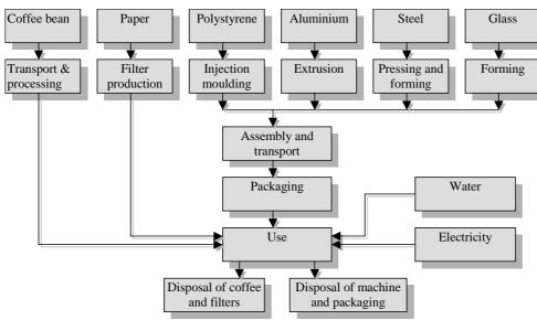
Figure 2: Example of a simplified process tree for the life cycle of a coffee machine.
