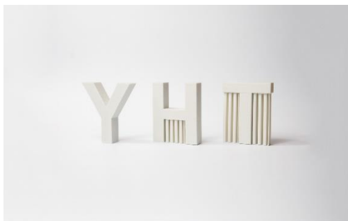
Figure 5 Supports en FDM
