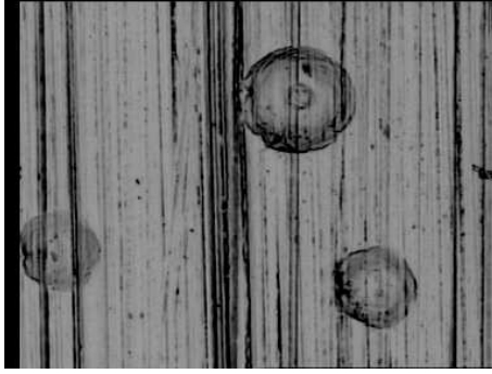
Figure 4.3 Picture of disk raceway tested with M50 particles ( magnification 40x), picture by F.Ville.
