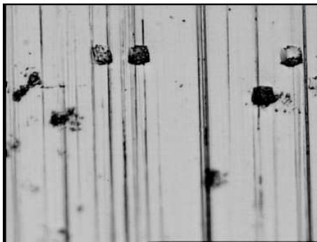
Figure 4.4 Picture of disk raceway tested with ACFTD (sand) (magnification 40x), picture by F.Ville.
