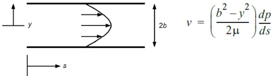
The resulting parabolic velocity profile in a wide rectangular channel is commonly called **Poiseuille flow**.
