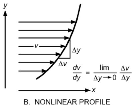
In **Newtonian fluids**, the rate of deformation proportional to the shearing stress
