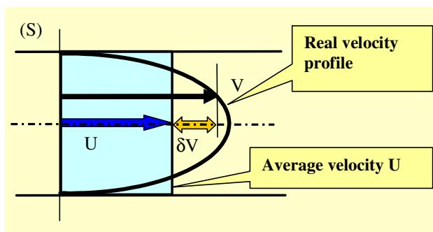
For laminar flow in a pipe,  $\alpha = 2$
