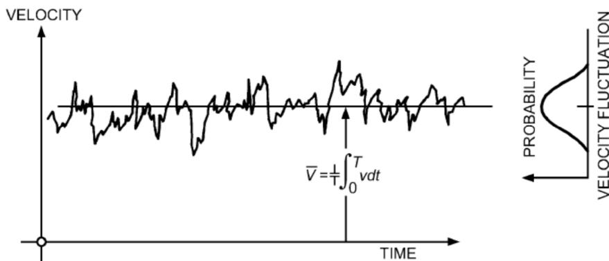
Turbulence can be quantified statistically.
