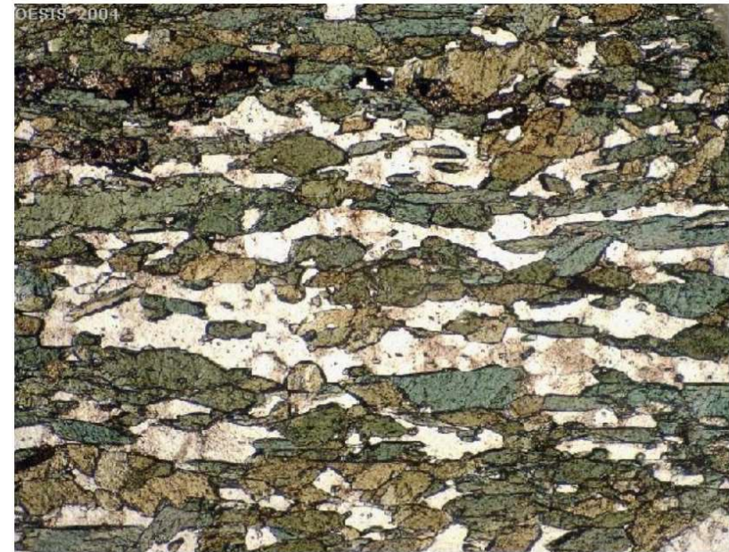
Amphibolite. This rock was originally a basic igneous rock (basalt or dolerite). When metamorphosed, the heating and compression changed the original minerals to hornblende (green) and feldspar (colourless), and gave the rock a banding of minerals. Field of view 2 mm.
